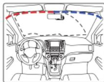
※Caution : few car navigations may face GPS reception of interruption. When installing Power cable and Rear cam connection cable. Recommend installing each cable in the opposite direction. For instance, Power cable is toward driver seat and rear cam connection cable is toward passenger seat.
